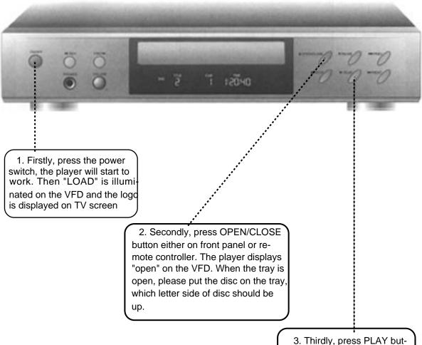
3. Thirdly, press PLAY button either on the front panel or remote controller, and the tray closes. The player will automatically read and identify the disc. Then the player will display the type and total time of the disc on the VFD, and begin to play.
